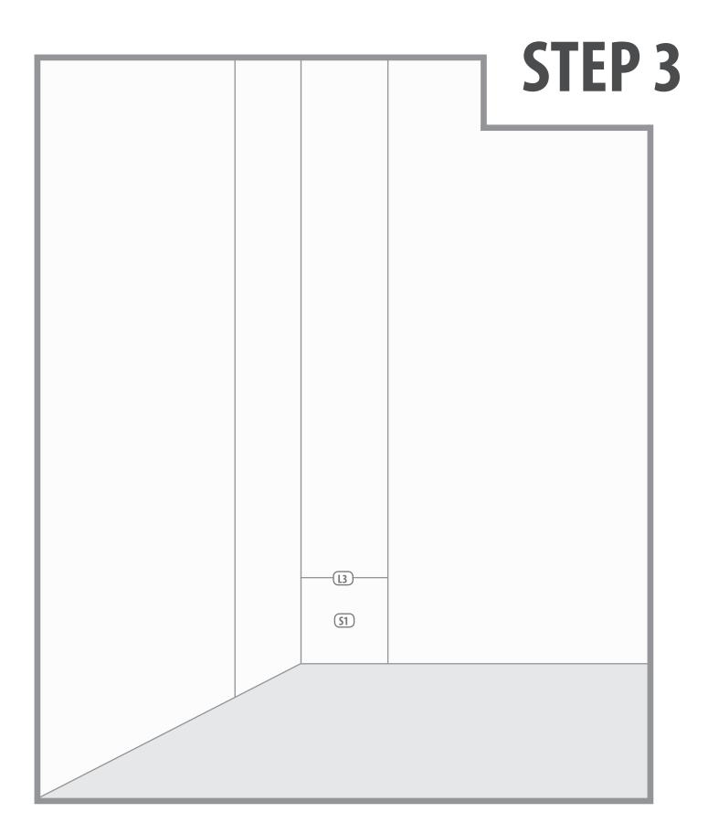
Using your hard graphite pencil, draw a line on the right wall of your corner parallel to the floor that creates a square with your corner edge, floor and L1. Label this line L3 and this square S1.
